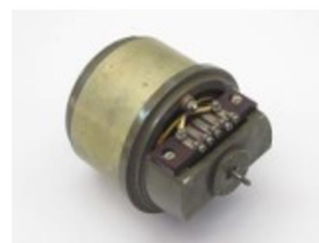
Obr. 5: Selsyn 55V, 50Hz
